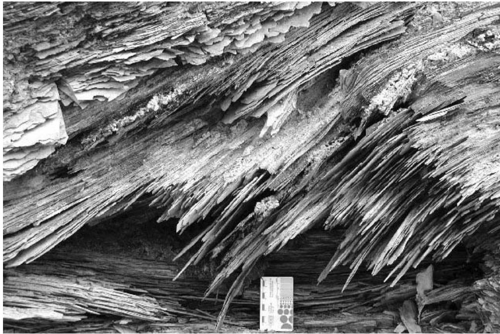
Figure 7 – Effects of pyrite oxidation in New Albany Shale, east of Elizabethton, Kentucky. Photo by Brandon Nuttall, Kentucky Geological Survey.
