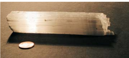
Figure E.4 - Fibrous gypsum crystal.
