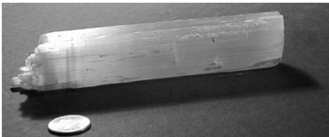
Figure 8 –Fibrous gypsum crystal (penny used for scale).
